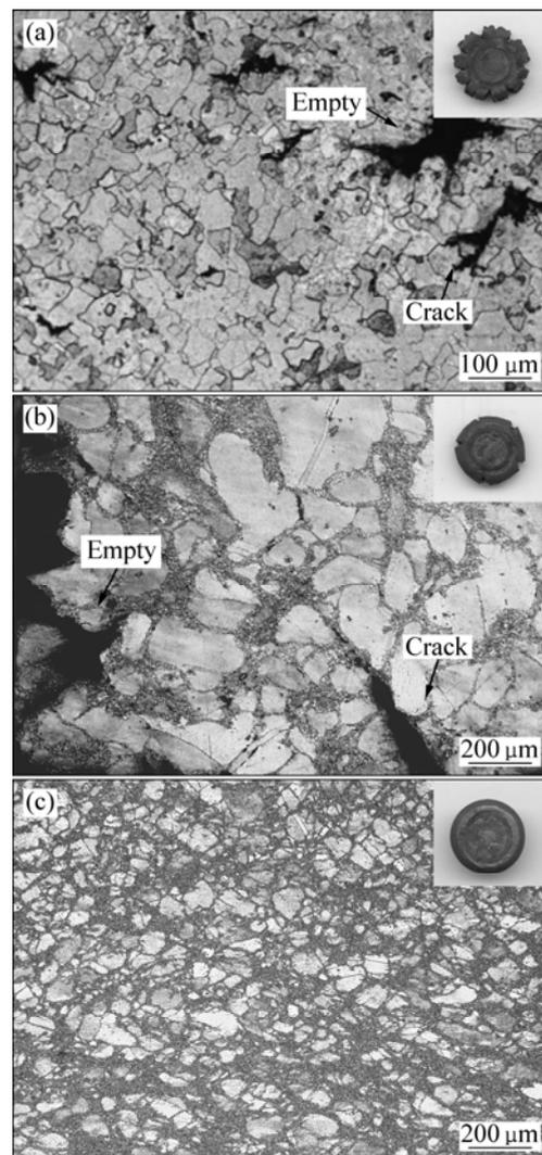
**Fig. 8** Microstructures of deformed specimens in different domains: (a)  $\dot{\epsilon}=10^{-3} \text{ s}^{-1}$ ,  $t=1150 \text{ }^{\circ}\text{C}$ ; (b)  $\dot{\epsilon}=10^{-1} \text{ s}^{-1}$ ,  $t=900 \text{ }^{\circ}\text{C}$ ; (c)  $\dot{\epsilon}=10^{-1} \text{ s}^{-1}$ ,  $t=1050 \text{ }^{\circ}\text{C}$
