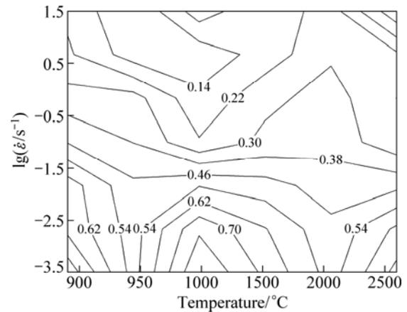
**Fig. 1** Power dissipation rate map at different strain rates and temperatures with a strain of 0.6
