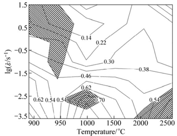
Fig. 3 Processing map of MALAS's instability criterion for GH79 superalloy
