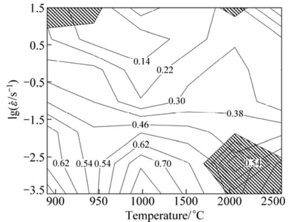
Fig. 6 Processing map of SEMIATIN’s instability criterion for GH79 superalloy
