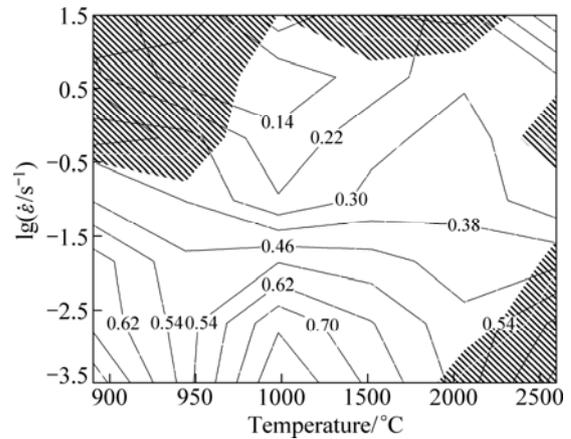
Fig. 5 Processing map of MURTY’s instability criterion for GH79 superalloy
