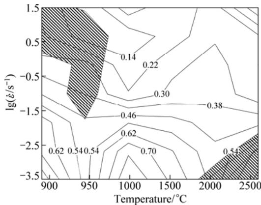
Fig. 2 Processing map of GEGEL's instability criterion for GH79 superalloy
