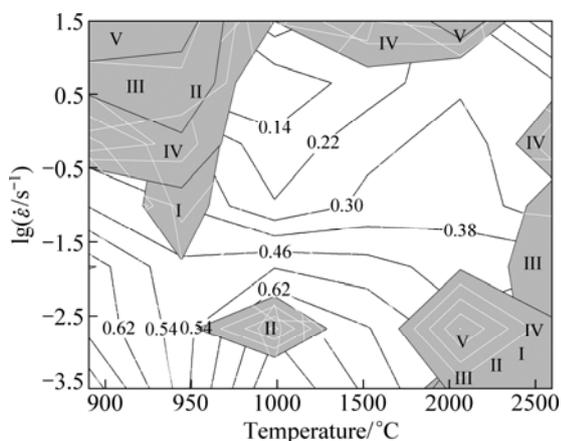
**Fig. 7** Instability maps through different instability criteria for GH79 superalloy: I—GEGEL; II—MALAS; III—PRASAD; IV—MURTY; V—SEMIATIN
