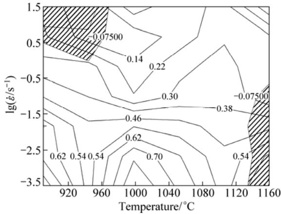
Fig. 4 Processing map of PRASAD’s instability criterion for GH79 superalloy
