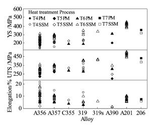
Fig.4 Tensile properties of SSM aluminum alloys compared with permanent mould (PM) cast ones
