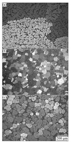
**Fig.9** Grains structure of cast C355 (a), forged 2618 (b) and SSM 319s (c), indicating comparable grain size between forged and SSM alloys, while both significant finer than cast alloy
