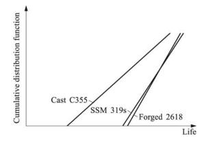
**Fig.8** SSM 319s compressor wheel showing superior durability over cast C355 compressor wheel while comparable with forged 2618
