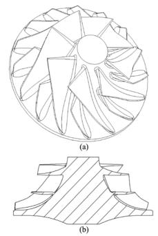
Fig.3 Overview (a) and section view (b) of typical compressor wheel
