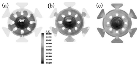
**Fig.10** CFD simulation showing temperature distribution for die filling: (a)  $t=0.1083$  s; (b)  $t=0.1123$  s; (c)  $t=0.1174$  s
