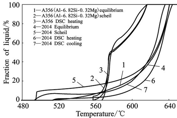
Fig.5 Curves of liquid fraction vs temperature[17]
