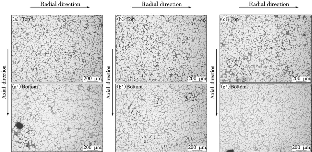
**Fig.7** Microstructures of billet at different location after three step induction heating at 25 kW along axial direction and radial directions: (a),(a') R-core; (b), (b') Middle; (c), (c') Edge
