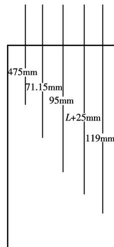
**Fig.4** Location of thermocouples in billet during induction heating
