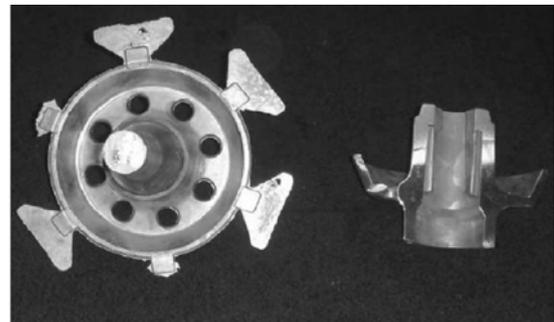
**Fig.11** Sample photographs of thixocast component
