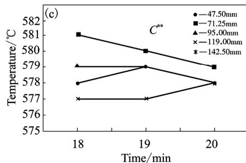
Fig.6 Temperature profiles of thermocouples located at different positions in billet during three step induction heating process at 25 kW
