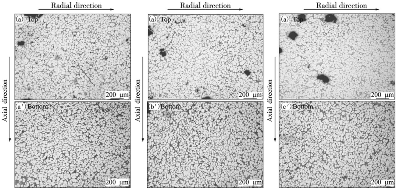
**Fig.9** Microstructures of billet at different locations after three step induction heating 50 kW along axial as well as radial directions: (a),(a') R-core; (b), (b') Middle; (c), (c') Edge
