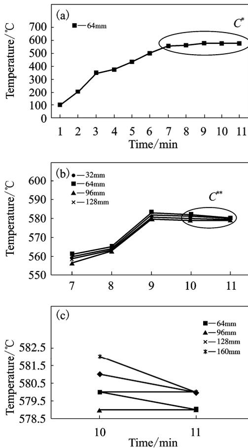
**Fig.8** Temperature profiles of thermocouples located at different positions in billet during three step induction heating process at 50 kW
