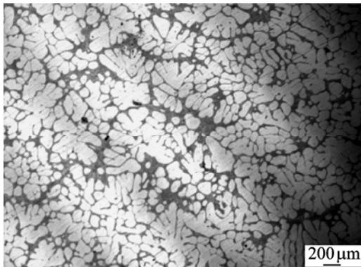
**Fig.3** Microstructure of electromagnetic stirred billet at 350A, 50 Hz before induction heating
