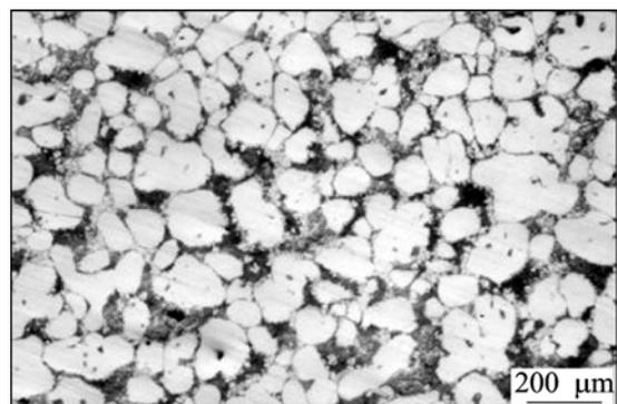
**Fig.12** Microstructure of semisolid cast component
