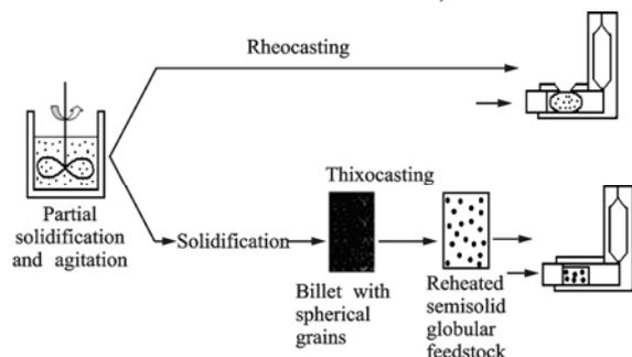
**Fig.1** Classification of semisolid processes
