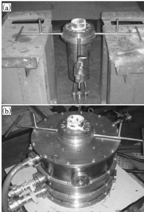
**Fig.2** Photographs of metallic mould(a) and electromagnetic stirrer(b)
