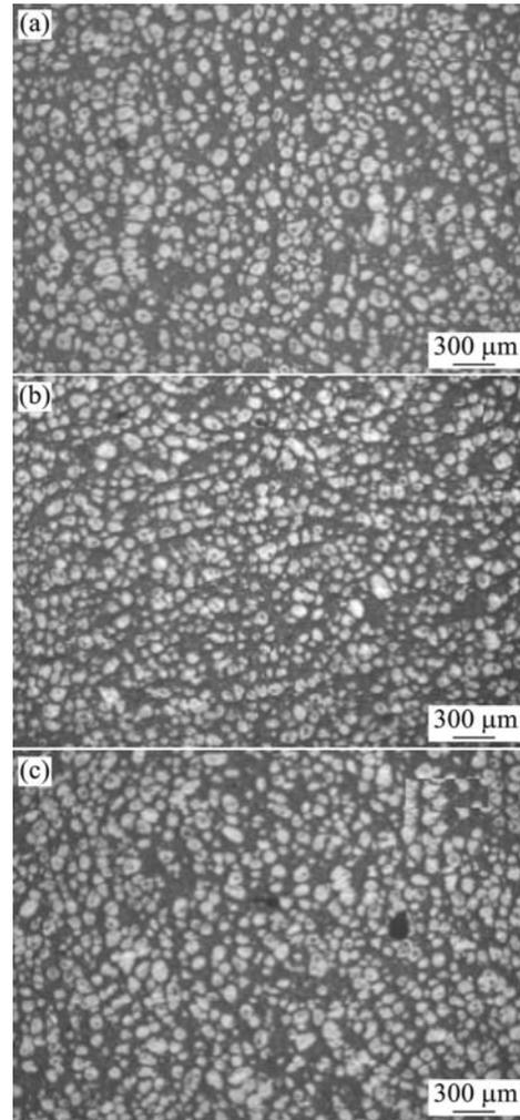
Fig.5 Microstructures of sampling location (vertical section through diameter) at 828 K for 30 min
