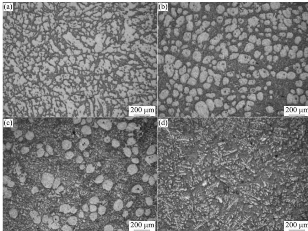
**Fig.3** Effect of heating temperature on microstructures (middle section): (a) 823 K; (b) 828 K; (c) 833 K; (d) 838 K
