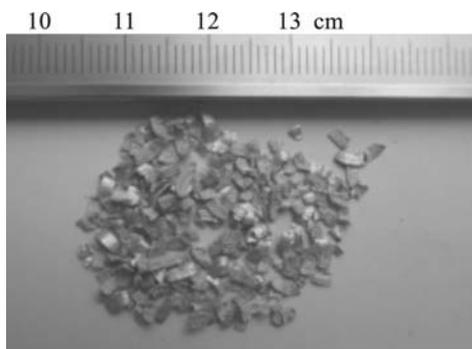
**Fig.1** Appearance of machined ADC12 chips
