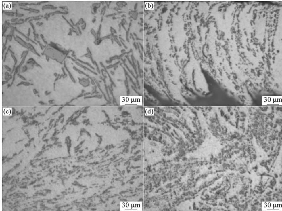
**Fig.2** Typical optical micrographs: (a) Cast piece; (b) Chips; (c) Compact chips under 400 MPa at room temperature (middle section); (d) Compact chips under 400 MPa after heat-treatment at 473 K for 20 min (middle section)
