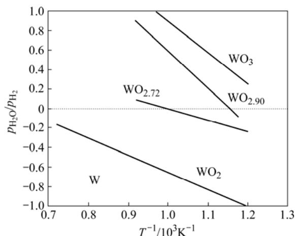
Fig.3 Equilibrium curves of different tungsten oxides and tungsten
