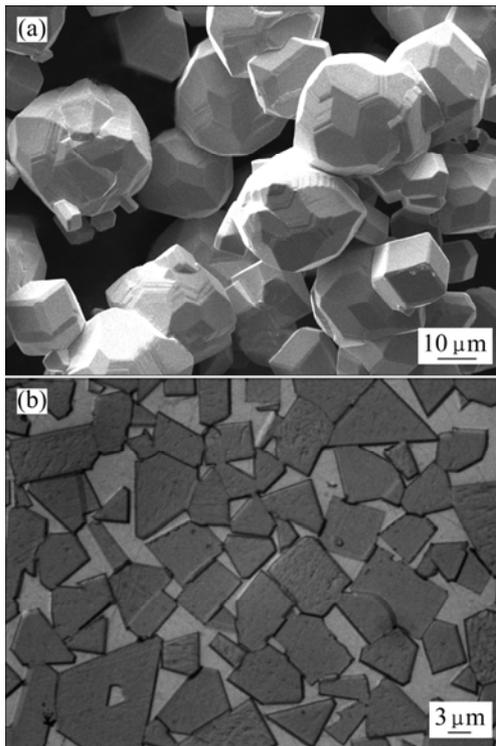
**Fig.4** Morphologies of coarse-grain tungsten (a) and WC-Co alloy (b)
