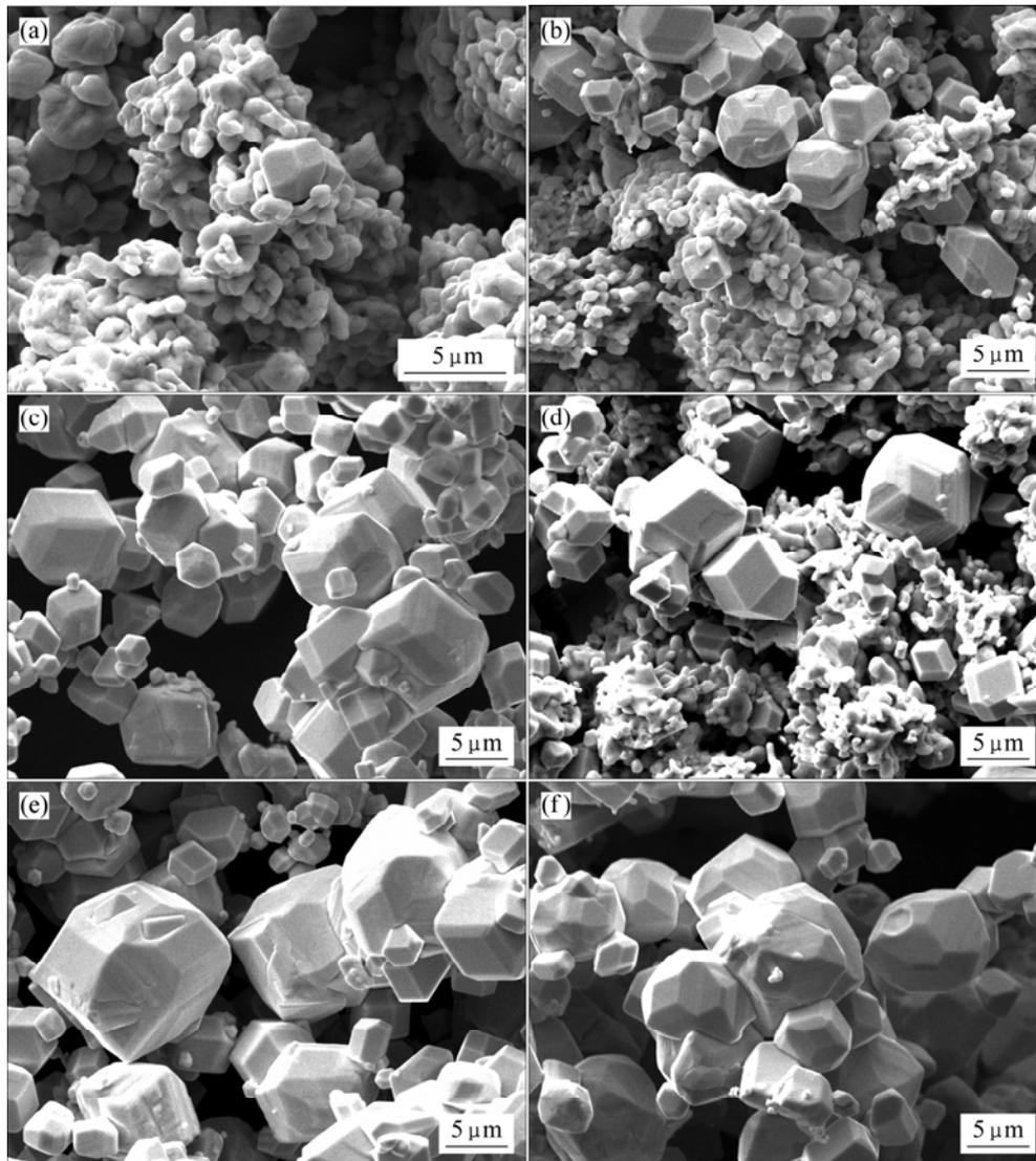
**Fig.1** Morphologies of powder in boat N6(a), N7(b), N9 top layer(c), N9 middle layer (d), N10 middle layer(e) and N10 bottom layer(f)
