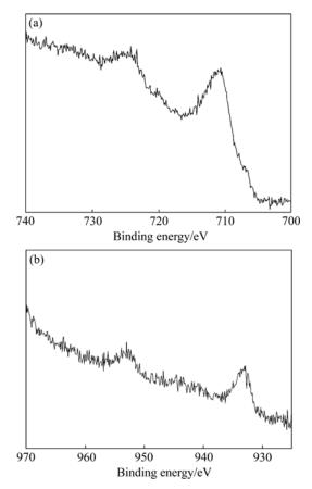
**Fig.7** XPS analysis of worn surface lubricated with 50CC oil+0.2% Cu: (a) Fe 2p; (b) Cu 2p
