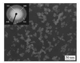
Fig.1 TEM image and ED pattern of Cu nanoparticles
