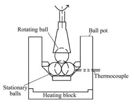
Fig.2 Schematic diagram of four-ball tester
