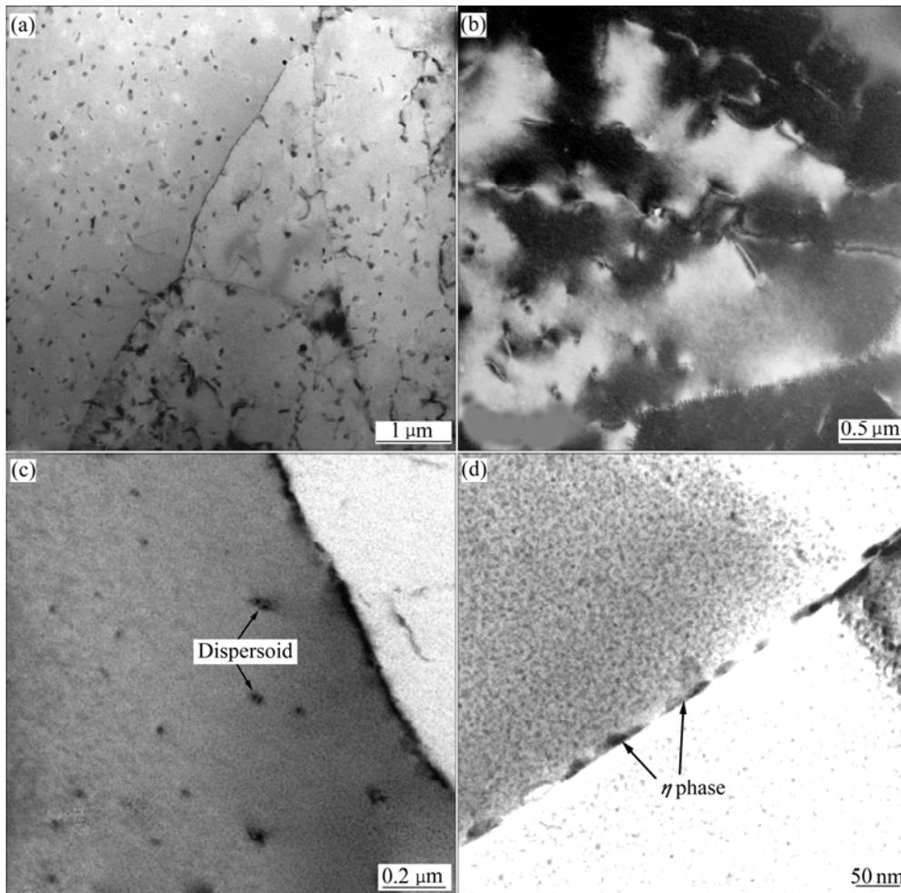
**Fig.4** TEM images of T6-tempered Al-Zn-Mg-Cu-Zr alloy (7A60+Yb)
