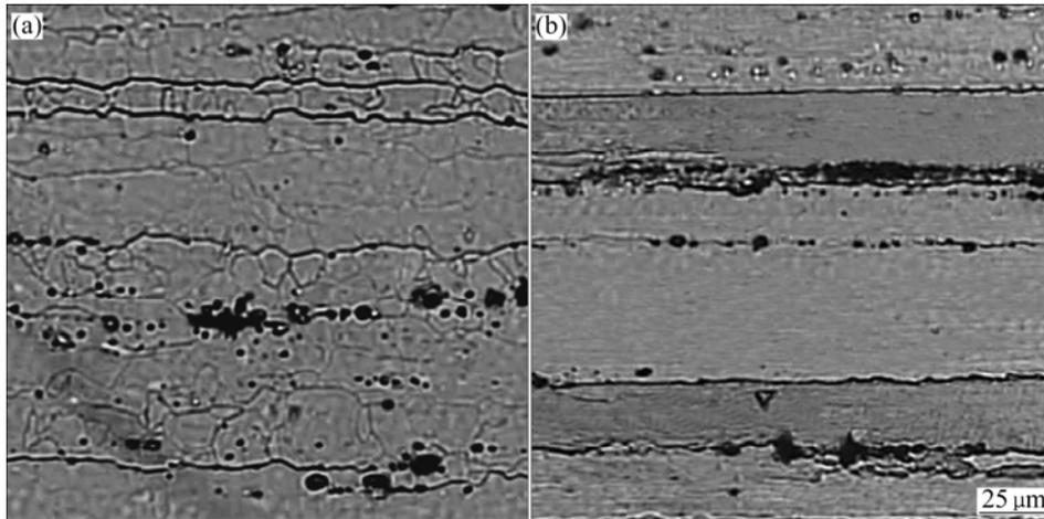
**Fig.3** Optical microstructures of two studied alloys with T6 ageing treatment: (a) 7A60-1; (b) 7A60+Yb-1
