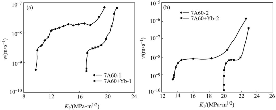
**Fig.1** Relationships between SCC growth rate and stress intensity factor in dropwise 3.5% NaCl environment for 7A60 alloys with Yb addition in different ageing treatments: (a) T6; (b) T77
