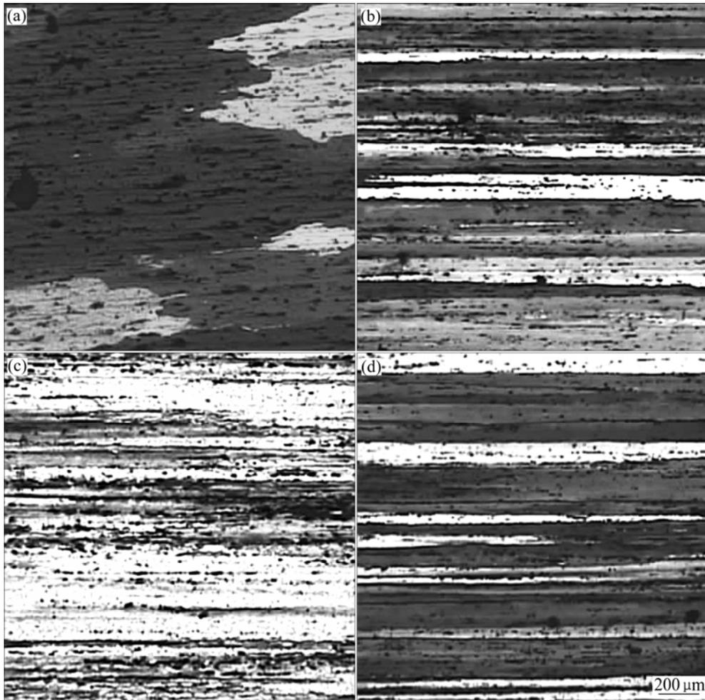
**Fig.2** Optical microstructures of two studied alloys with solution treatment: (a) 7A60-1(L-T surface); (b) 7A60+Yb-1(L-T surface); (c) 7A60-1(L-S surface); (d) 7AYb+Yb-1(L-S surface)
