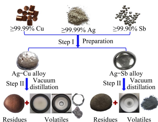
Fig. 1 Experimental procedure including original materials, alloy samples, and products after vacuum distillation
