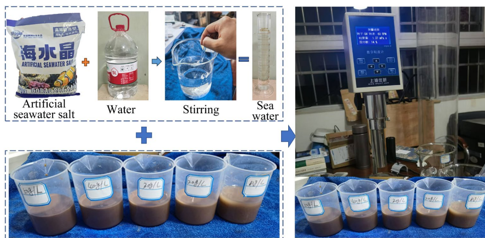
Fig. 7 Viscosity test process of sediment solutions with different concentrations
