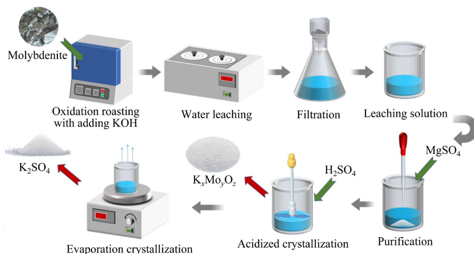
Fig. 2 Schematic diagram for molybdenum recovery from molybdenite
