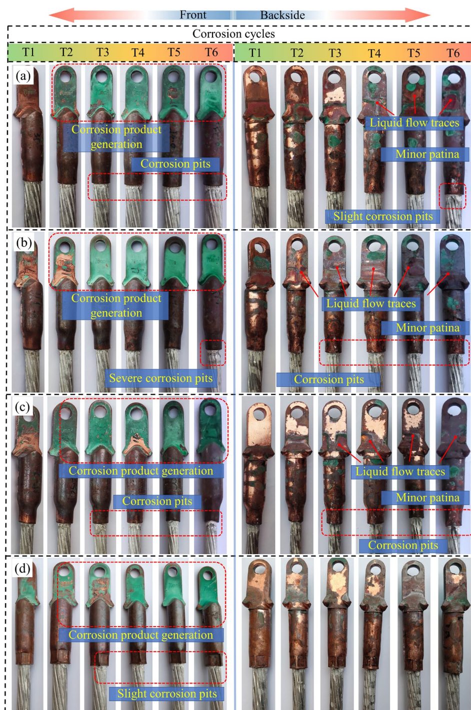
Fig. 4 Macroscopic morphology of cable joints with different corrosion cycles on both sides: (a) Type I; (b) Type II; (c) Type III; (d) Type IV
