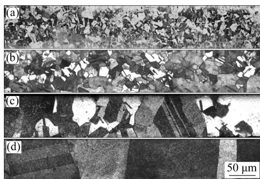
Fig. 1 Microstructures of samples with different grain sizes: (a) 3.3 \mu\text{m} ; (b) 7.7 \mu\text{m} ; (c) 23.2 \mu\text{m} ; (d) 75.2 \mu\text{m}
