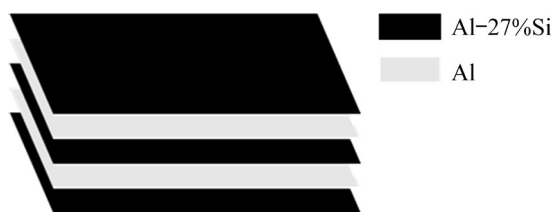
Fig. 1 Schematic diagram of Al/Al–27%Si laminated composite structure
