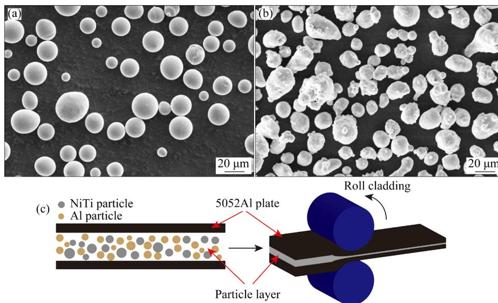
**Fig. 1** SEM images of NiTi particles (a) and Al particles (b), and schematic diagram of rolling process (c)
