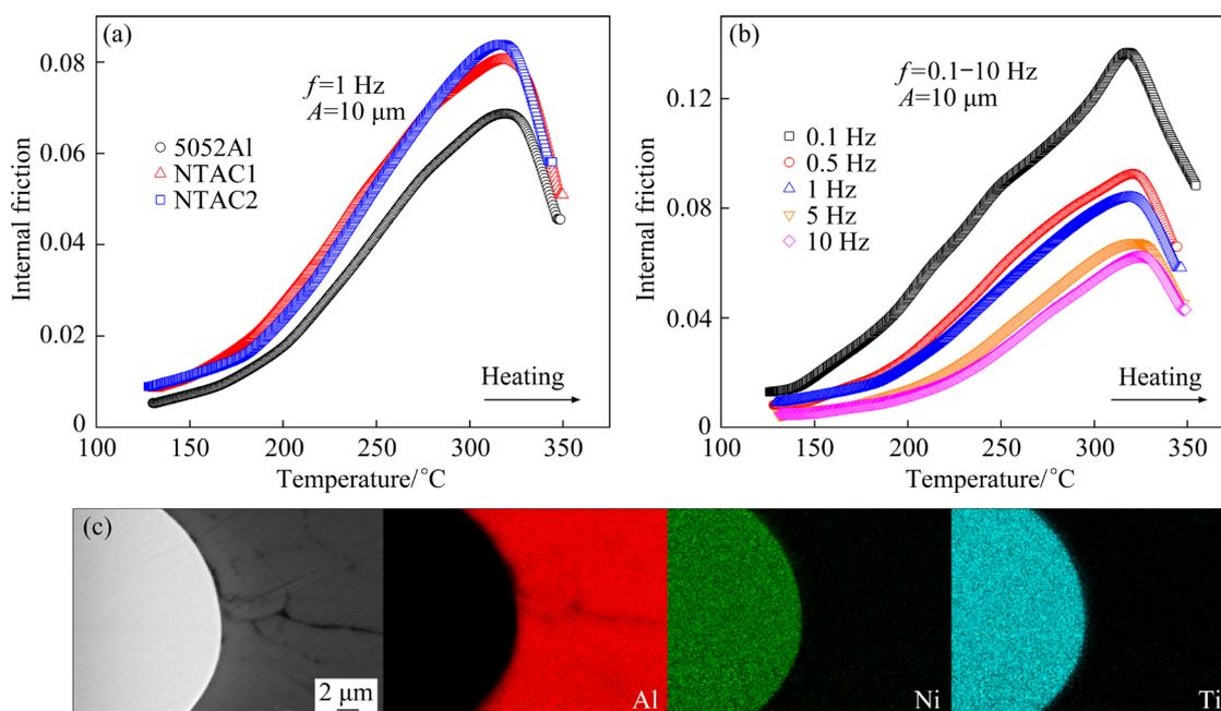
**Fig. 8** Internal friction–temperature curves of laminated composites and 5052Al alloy at 120–360 °C (a), internal friction–temperature curves of NTAC2 samples at different test frequencies (b), and SEM image of NTAC2 sample after high-temperature damping test and area scanning element distribution maps (c)
