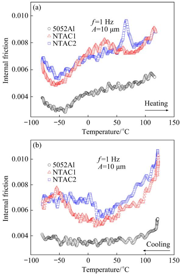
**Fig. 9** Internal friction–temperature curves of laminated composites and 5052Al alloy within range of  $-80$  to  $120$  °C: (a) Heating process; (b) Cooling process
