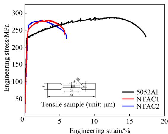
**Fig. 5** Engineering stress–strain curves of laminated composites and 5052Al alloy
