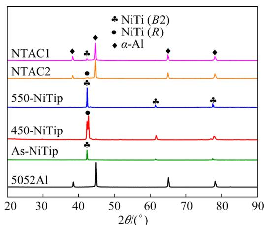
**Fig. 3** XRD patterns of 5052Al alloy, NiTi particles and laminated composites
