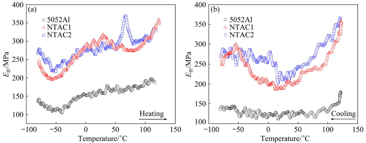
**Fig. 11**  $E_{IF}$ –temperature curves of laminated composites and 5052 Al alloy: (a) Heating process; (b) Cooling process
