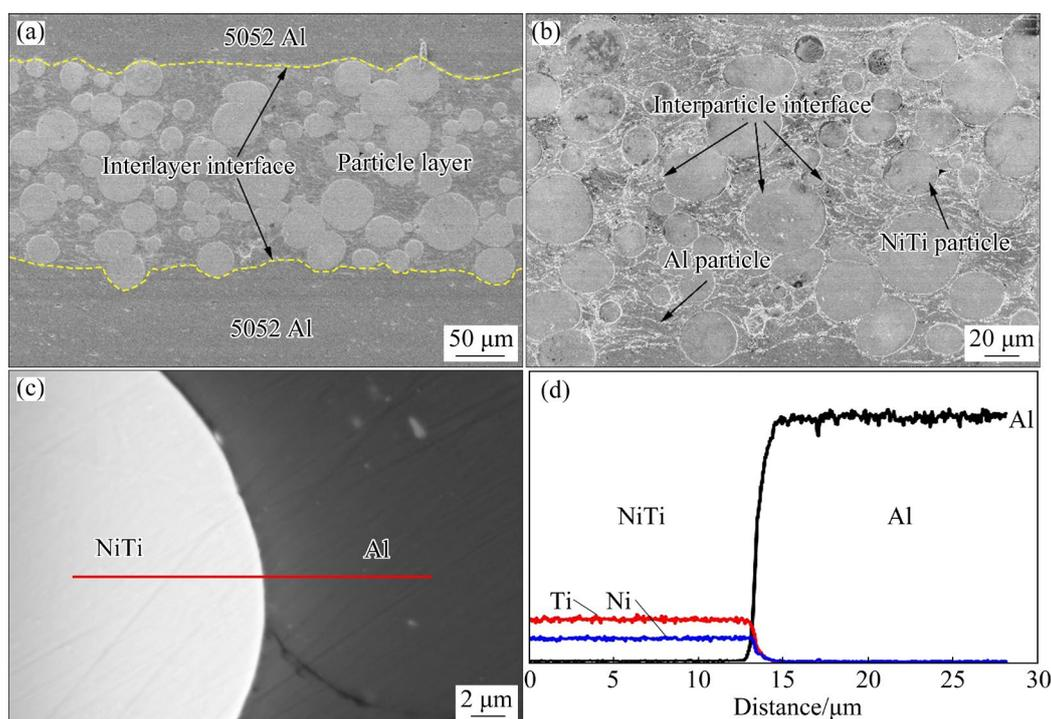
**Fig. 2** SEM images of NTAC1 sample: (a) Morphology of corroded sample; (b) Local enlarged view in (a); (c) Morphology of uncorroded sample; (d) Scanning element distribution of line in (c)
