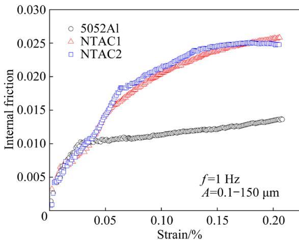
**Fig. 7** Internal friction–strain curves of laminated composites and 5052Al alloy
