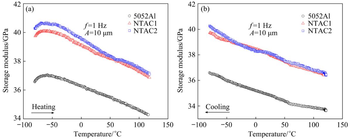
**Fig. 10** Storage modulus–temperature curves of laminated composites and 5052Al alloy in range of –80 to 120 °C: (a) Heating process; (b) Cooling process
