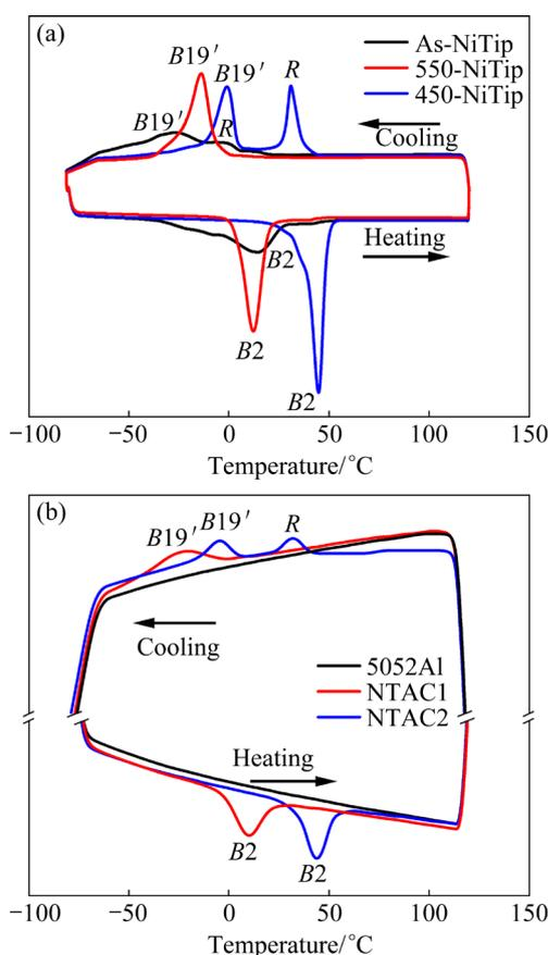
**Fig. 4** DSC curves of samples: (a) NiTi particles with different aging states; (b) Laminated composites and 5052Al alloys
