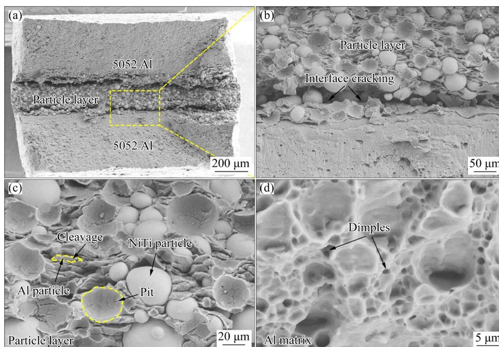
**Fig. 6** Fracture morphology of NTAC1 sample: (a) Overall morphology; (b) Local amplification of (a); (c) Granular layer; (d) Aluminum matrix
