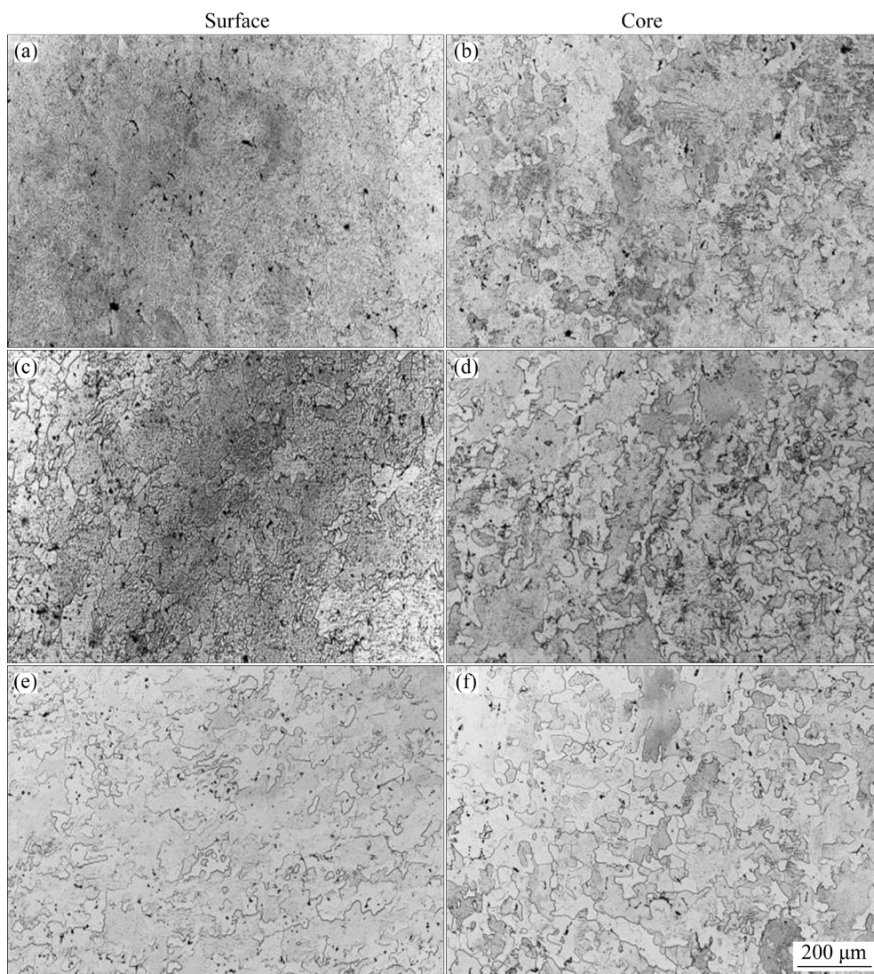
Fig. 2 Metallographic images of aluminum forgings after SCPD and solution treatment at 470 °C for different durations: (a, b) 10 min; (c, d) 30 min; (e, f) 60 min
