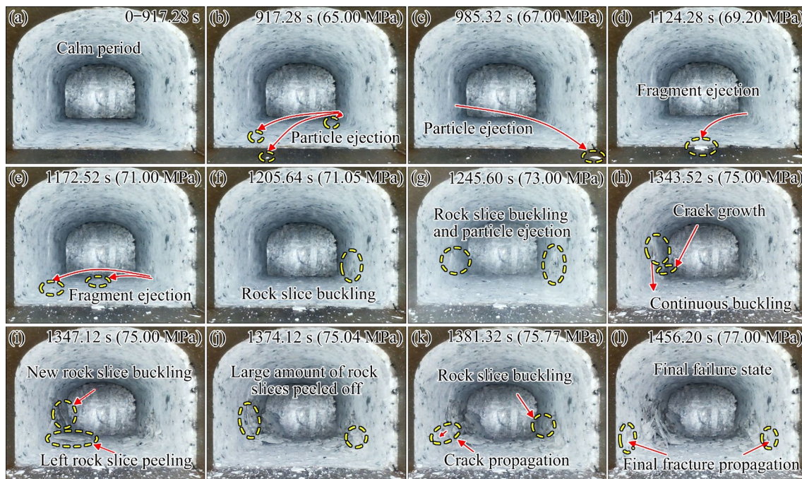
Fig. 6 Failure process images of Specimen T-10-30
