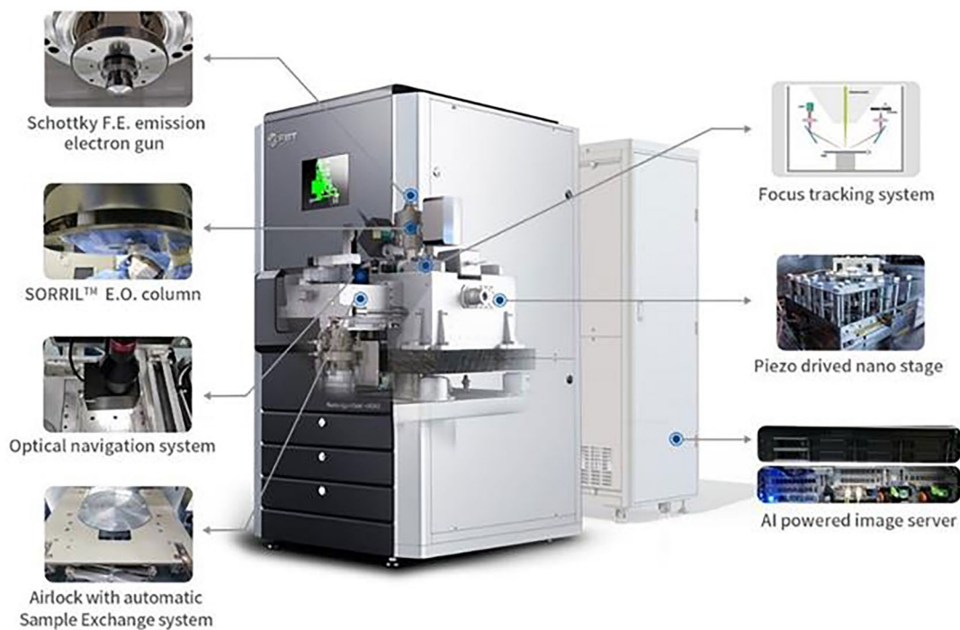
Fig. 16 System components in Navigator-100 high-throughput SEM [74]
