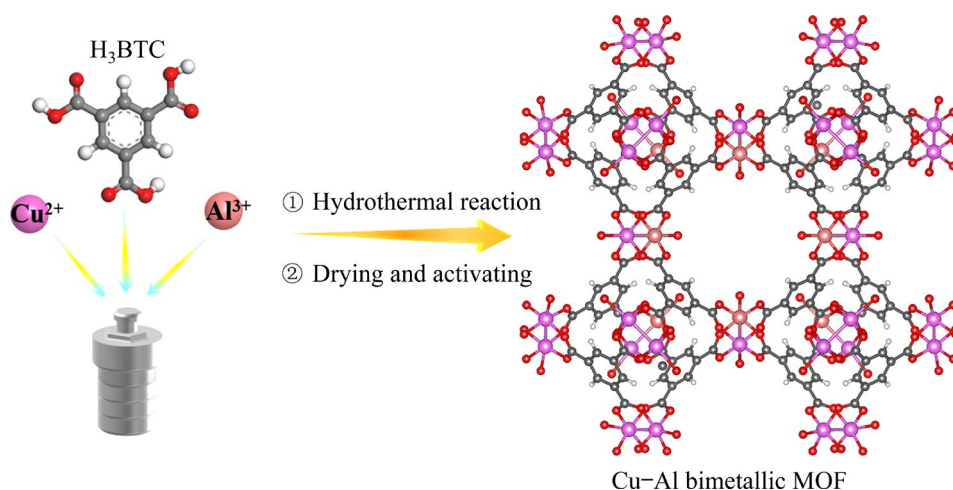
Fig. 1 Schematic diagram of fabrication of Cu–Al bimetallic MOF
