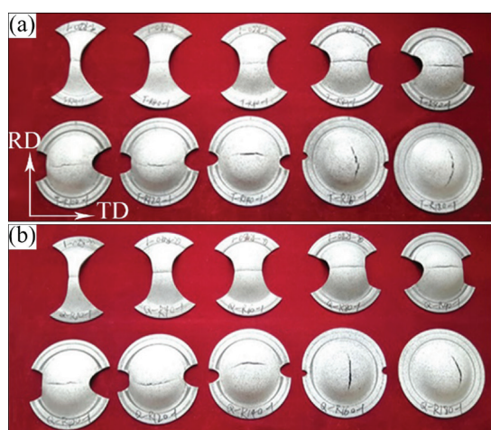
Fig. 3 Bulging specimens: (a) Group A; (b) Group B
