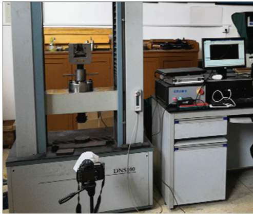
Fig. 5 Uniaxial compression test equipment of rock with three non-parallel cracks
