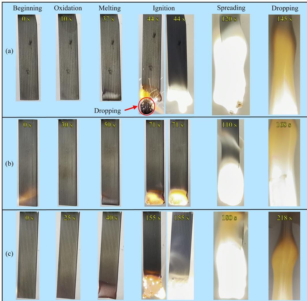
**Fig. 3** Fire progresses of ZM5 (a), ZM6 (b) and WE43 (c) Mg alloy samples with dimension of 3 mm × 20 mm × 100 mm
