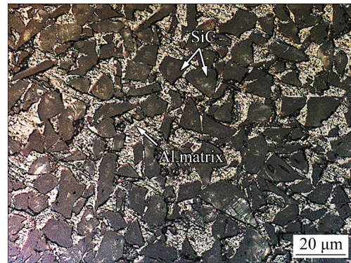
Fig. 1 Metallographic microstructure of 60vol.%SiC p /Al MMC
