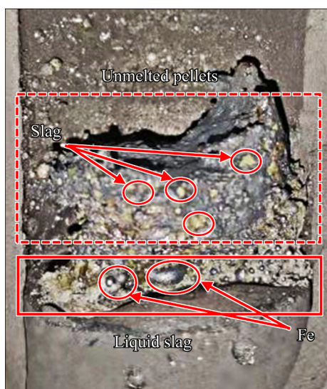
Fig. 7 Photograph of unmelted pellets after melting for 7.5 min
