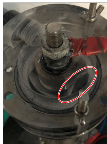
Fig. 7 Deposited indium in electrolytic cell at flow rate of 500 L/h
