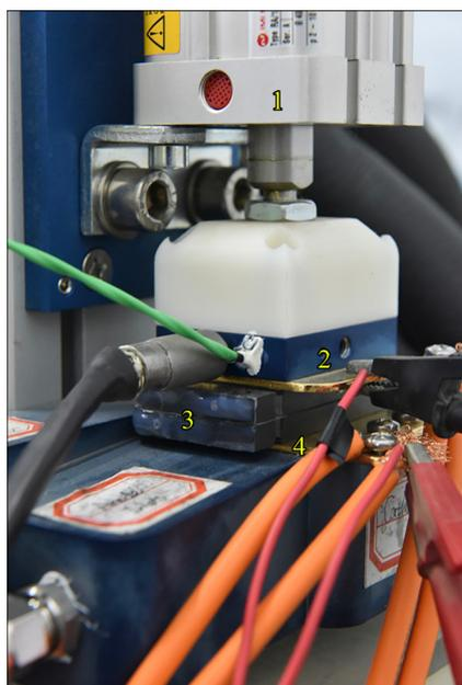
**Fig. 9** Experimental proton exchange membrane fuel cell (PEMFC) construction: 1—Nitrogen gas pressure pump; 2—Anode heating plate ( $H_2$ ); 3—Membrane electrode assemblies; 4—Cathode heating plate (Air)
