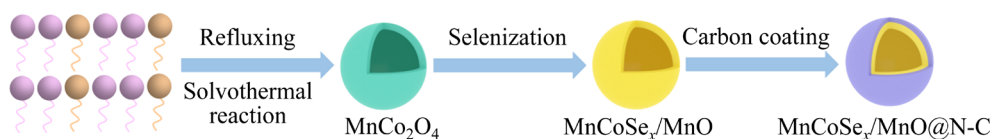
Fig. 1 Schematic illustration for synthesis of hollow MnCoSe x /MnO@N-C nanospheres
