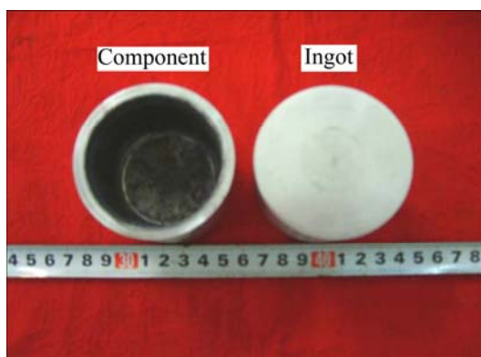
Fig. 11 AZ91D magnesium alloy components thixoformed from starting produced by SIMA route
