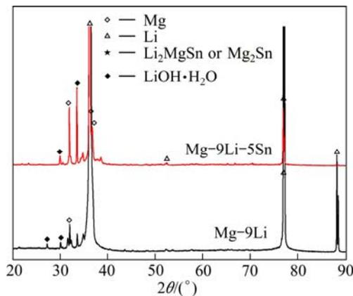
**Fig. 5** XRD patterns of as-extruded Mg-9Li-*x*Li alloys (LiOH·H<sub>2</sub>O was also observed. Its existence does not disturb the observation)
