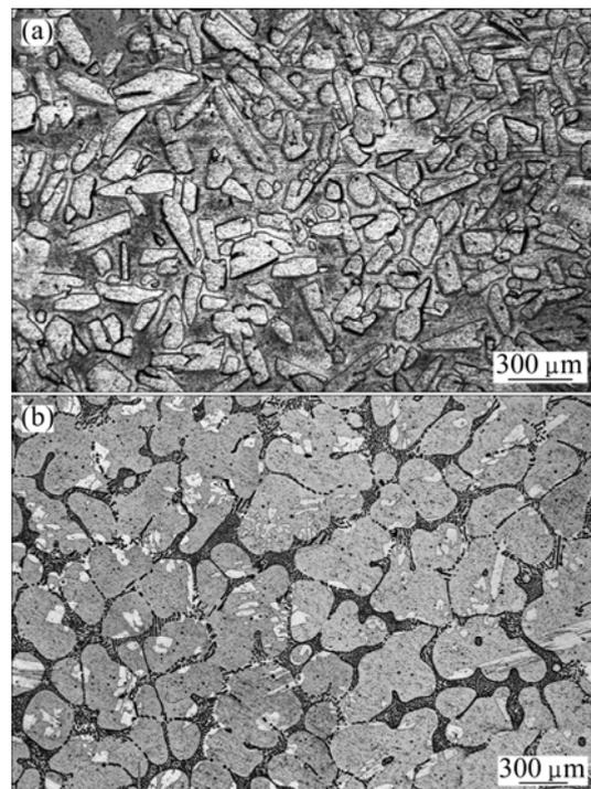
**Fig. 1** Optical microstructures of as-cast alloys: (a) Mg–9Li alloy; (b) Mg–9Li– $x$ Sn alloy
