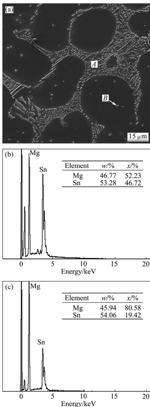
Fig. 2 SEM image of as-cast Mg-9Li-5Sn alloy (a) and corresponding EDS spectra of point A (b) and point B (c)
