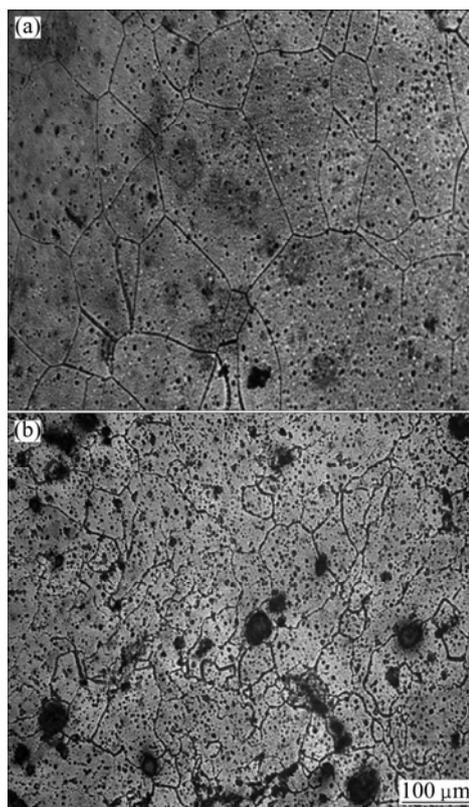
Fig. 4 Microstructure of as-extruded Mg-9Li alloy (a) and Mg-9Li-5Sn alloy (b)
