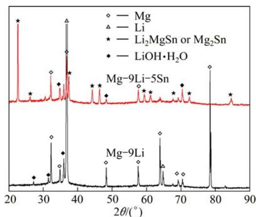
Fig. 3 XRD patterns of as-cast Mg-9Li-xLi alloy (LiOH·H<sub>2</sub>O was observed in the XRD result because Li is highly chemical activity and is easy to react with H<sub>2</sub>O during the sample preparation. Basically, its existence does not disturb the observation)
