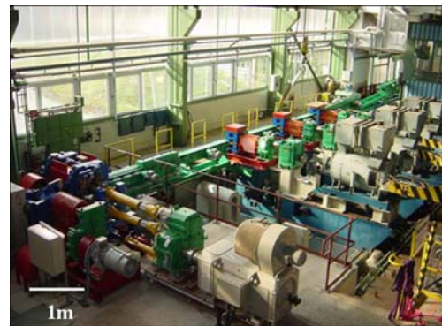
Fig. 1 Complete view of pilot high-speed continuous rod rolling mill at University of Freiberg in Germany
