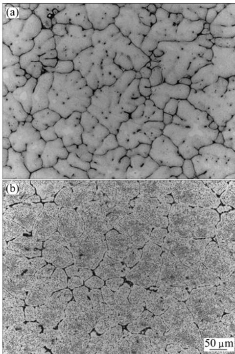
**Fig. 1** Optical microstructures of as-cast (a) and as-homogenized (b) 7055 alloy
