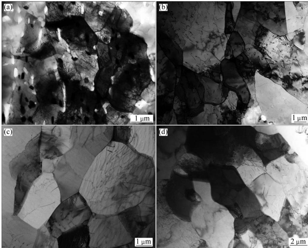
**Fig. 4** TEM images of samples deformed at different temperatures: (a) 300 °C; (b) 350 °C; (c) 400 °C; (d) 450 °C
