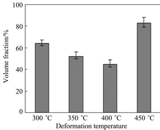
**Fig. 6** Recrystallization volume fraction of heat-treated 7055 alloy
