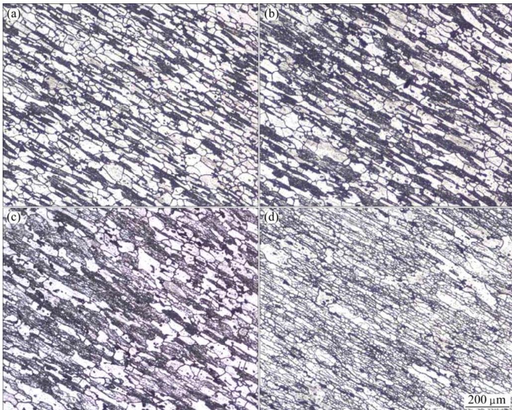
**Fig. 5** OM images of 7055 alloy deformed at various temperatures and same heat-treatment condition: (a) 300 °C; (b) 350 °C; (c) 400 °C; (d) 450 °C
