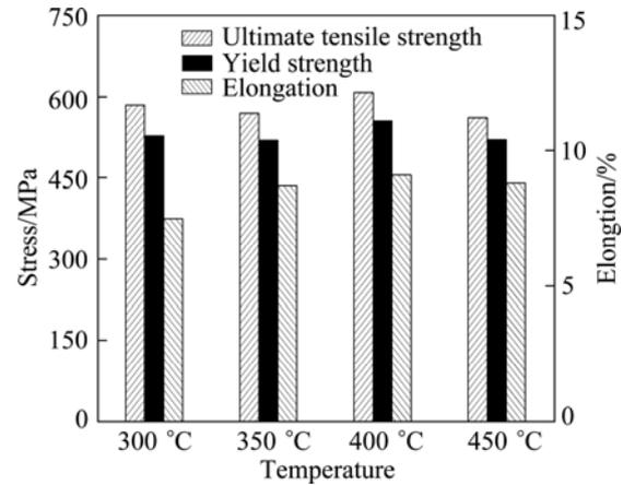
**Fig. 7** Mechanical properties of 7055 alloy deformed at various temperatures after heat treatment
