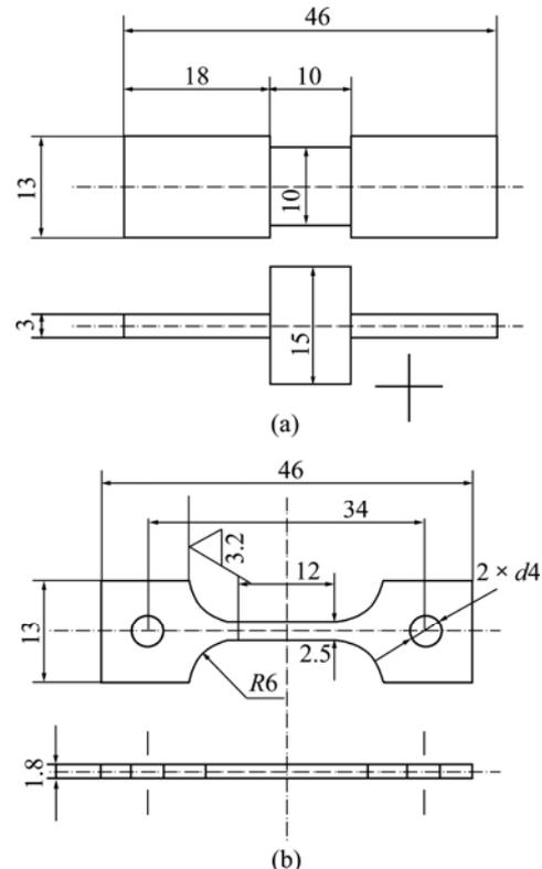
**Fig. 2** Schematic diagrams of hot-compressed sample (a) and tensile sample (b) (unit: mm)
