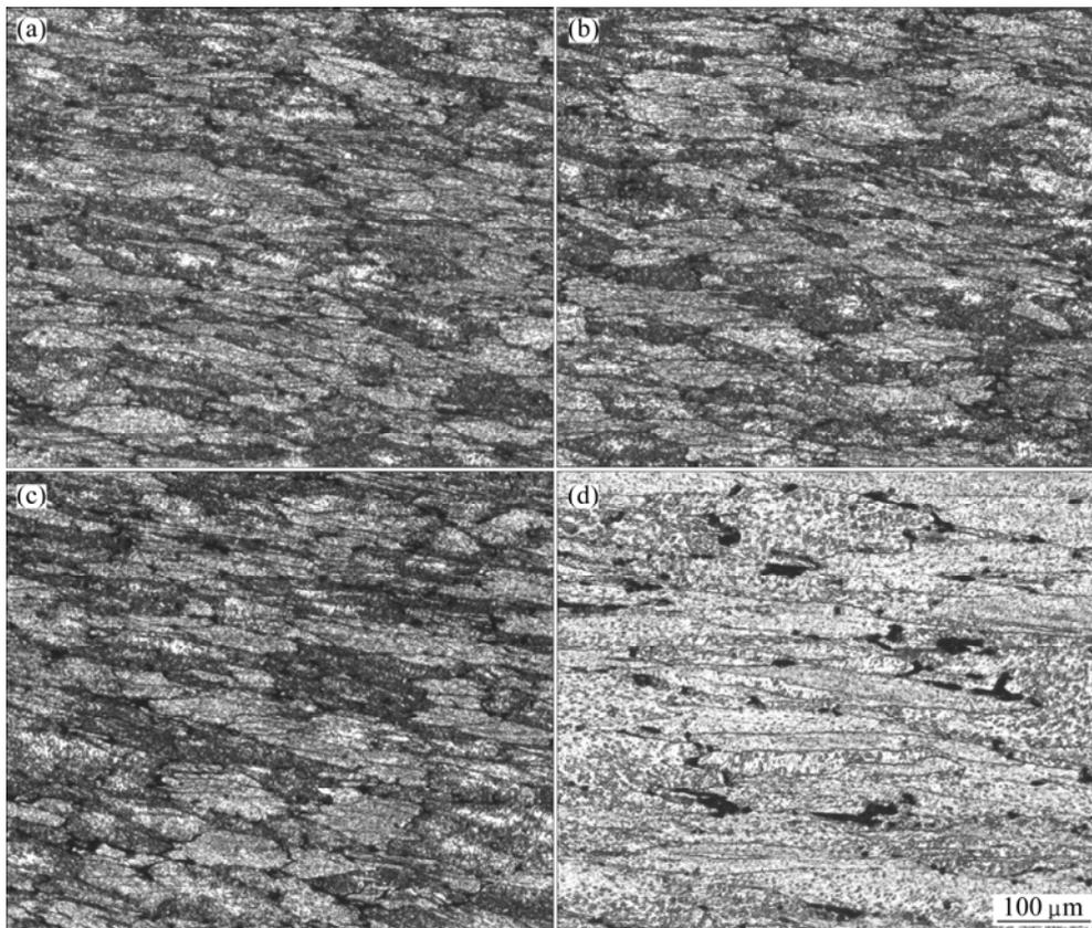
**Fig. 3** OM microstructures of samples deformed at different temperatures: (a) 300 °C; (b) 350 °C; (c) 400 °C; (d) 450 °C
