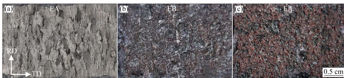
Fig. 9 Digital images showing surface morphology of samples after immersion in EXCO solution for 48 h: (a) 0Cu; (b) 1Cu; (c) 2.6Cu
