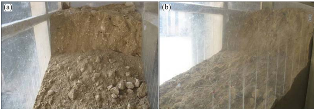
Fig. 9 Failure mode of soil talus-derived rock mass (no rainfall): (a) Front; (b) Side
