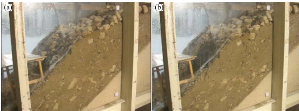
Fig. 4 Failure modes of framework talus-derived rock mass (rainfall): (a) Local slip collapse; (b) Large area of slump
