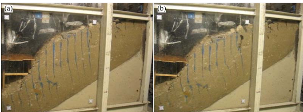
Fig. 10 Failure mode of soil talus-derived rock mass (rainfall): (a) Cracks appearing; (b) Cracks expanding
