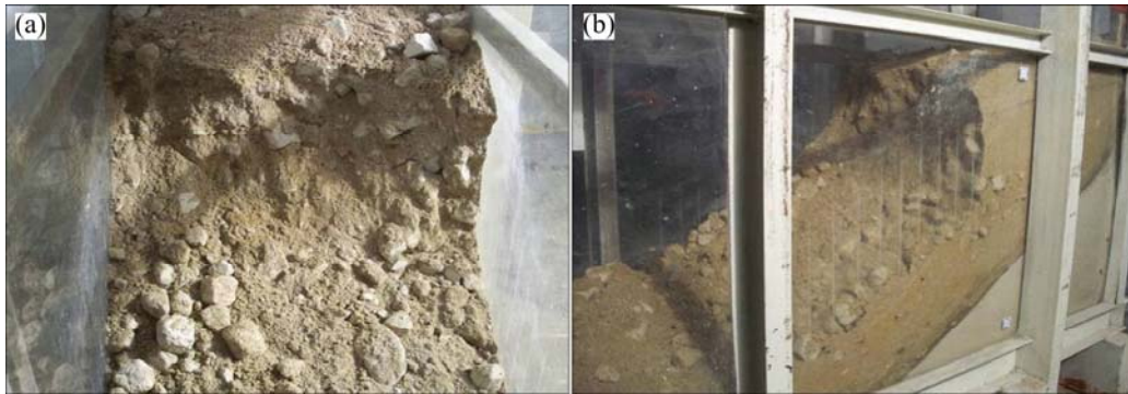
Fig. 7 Failure modes of suspension talus-derived rock mass (no rainfall): (a) Front; (b) Side
