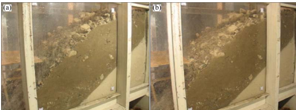
Fig. 6 Failure modes of filling-type talus-derived rock mass (rainfall): (a) Deformation development; (b) Slope toe sliding
