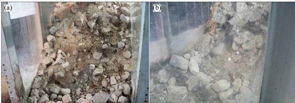
Fig. 5 Failure modes of filling-type talus-derived rock mass (no rainfall): (a) Front; (b) Side
