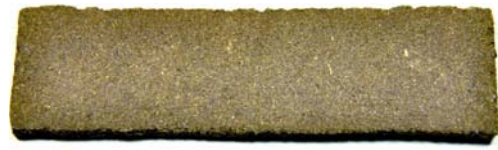
Fig. 2 Specimen made from palm oil sludge mixed with activated sludge cake by compression method
