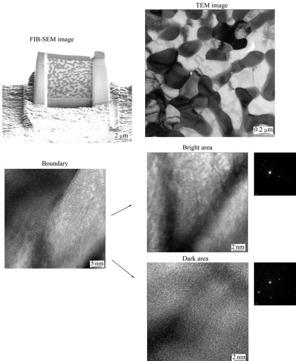
**Fig. 7** FIB-SEM and HR-TEM microstructures of eutectic composites sintered at 1500 °C for 30 min (Crystalline Al<sub>2</sub>O<sub>3</sub> appears dark and crystalline GdAlO<sub>3</sub> appears bright)
