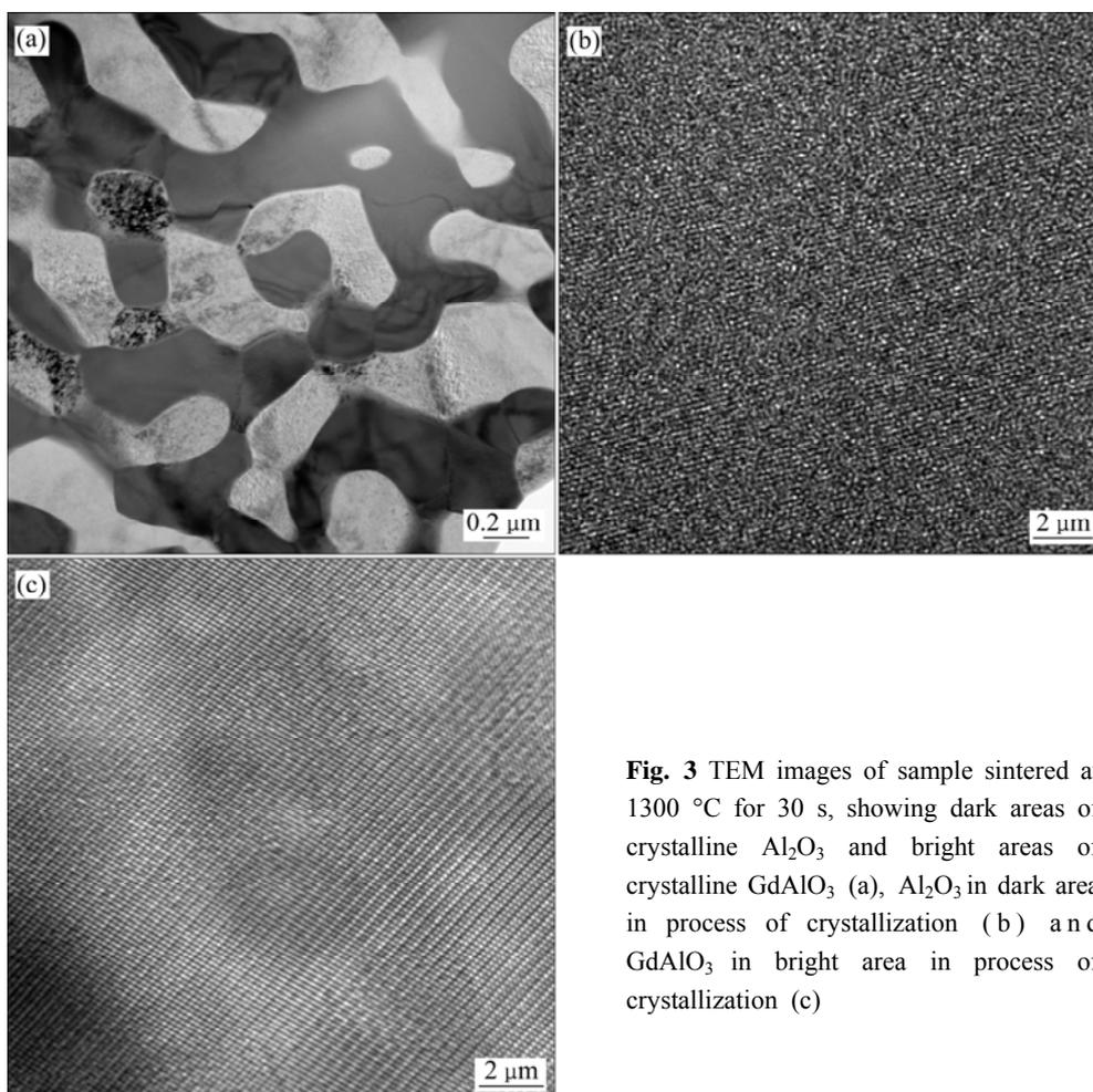
**Fig. 3** TEM images of sample sintered at 1300 °C for 30 s, showing dark areas of crystalline  $\text{Al}_2\text{O}_3$  and bright areas of crystalline  $\text{GdAlO}_3$  (a),  $\text{Al}_2\text{O}_3$  in dark area in process of crystallization (b) and  $\text{GdAlO}_3$  in bright area in process of crystallization (c)
