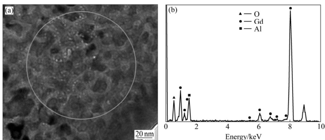
**Fig. 2** Region analyzed by EDS (a) and qualitative data with peaks for  $\text{GdAlO}_3$  identified (b)
