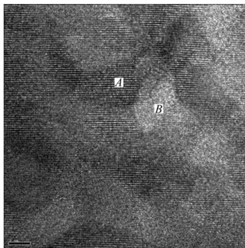
**Fig. 1** HR-TEM analysis of lattice image of eutectic 23% $\text{Gd}_2\text{O}_3$ -77% $\text{Al}_2\text{O}_3$  sintered at 1000 °C for 30 min
