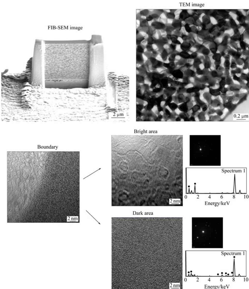
**Fig. 5** FIB-SEM and HR-TEM microstructures of eutectic composites sintered at 1500 °C for 2 min (Crystalline  $\text{Al}_2\text{O}_3$  appears dark and crystalline  $\text{GdAlO}_3$  appears bright)
