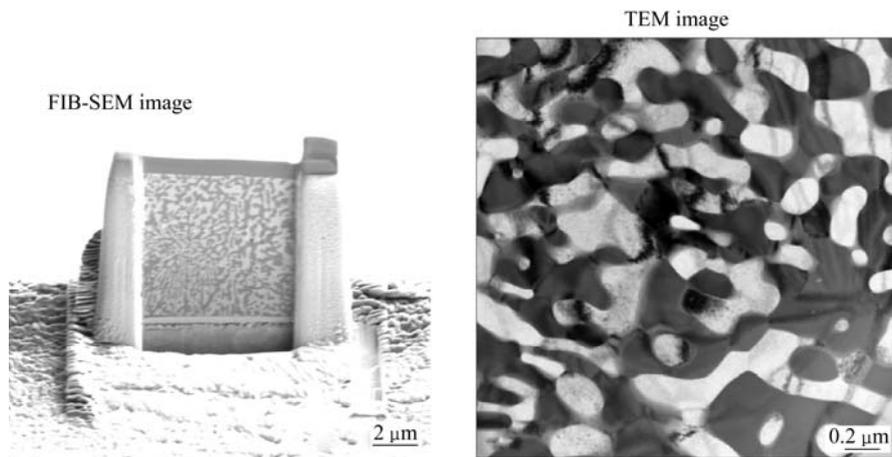
**Fig. 6** FIB-SEM and HR-TEM microstructures of eutectic composites sintered at 1500 °C for 8 min (Crystalline Al<sub>2</sub>O<sub>3</sub> appears dark and crystalline GdAlO<sub>3</sub> appears bright)
