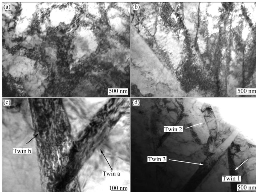
**Fig. 9** TEM images in DZ: (a) Dislocation cells; (b) Slab dislocations; (c, d) Interactions of twins
