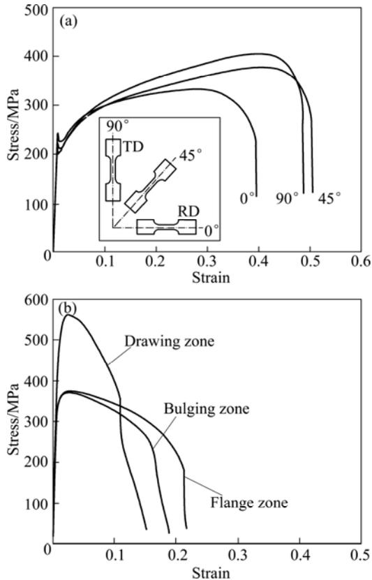
**Fig. 3** Uniaxial tension test of as-received CP-Ti sheet with illustration of sampling method (a) and drawn part (b)
