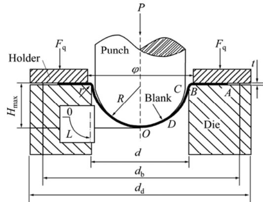
**Fig.1** Scheme of cold drawing-bulging of CP-Ti sheet with illustrations of deformation zones:  $AB$ —FZ;  $BC$ —Die corner;  $CD$ —DZ;  $DO$ —BZ;  $L$ —thickness measurement direction
