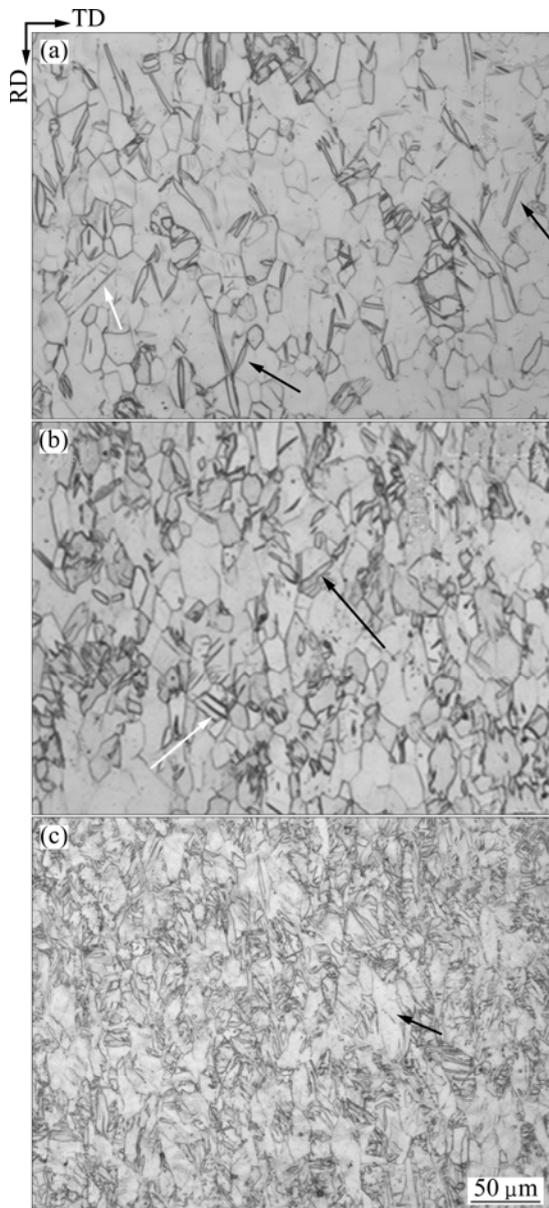
**Fig. 6** Optical microscopy images of samples in BZ (a), FZ (b) and DZ (c) of finished part with illustration of large-size twins by black arrows and small-size twins by white arrows
