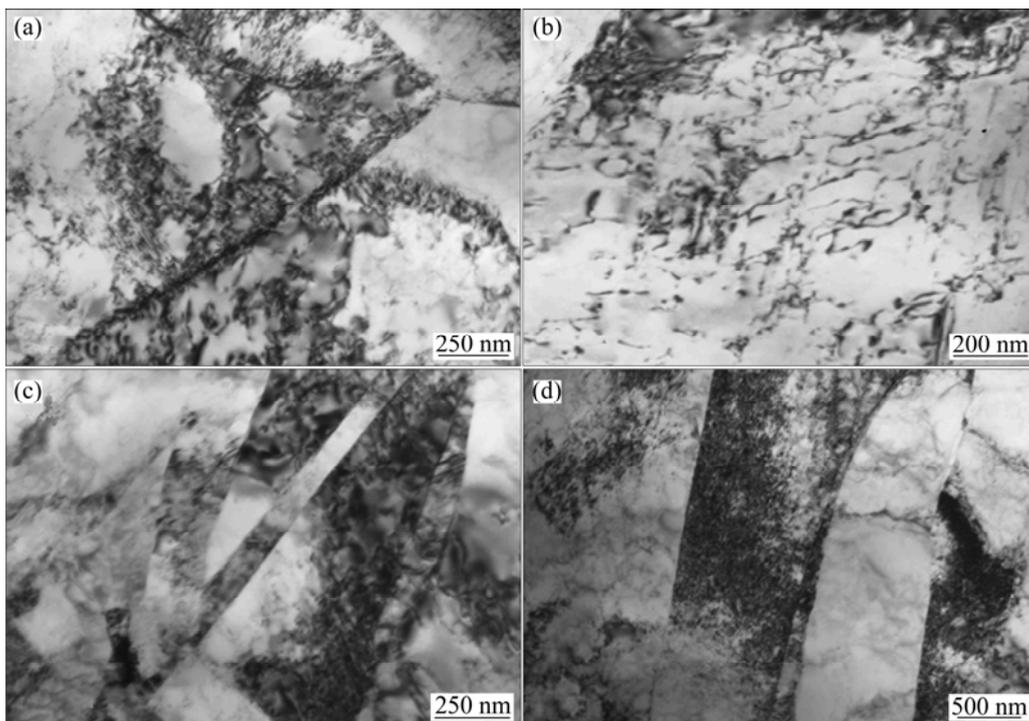
**Fig. 8** TEM images in FZ: (a) Dislocations at grain boundaries; (b) Dislocations within a grain; (c) Primary and secondary twins; (d) Parallel twins
