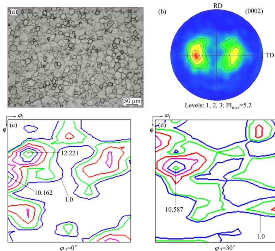
**Fig. 2** Microstructure (a), (0002) pole figure (b) and ODF sections (c, d) of as-received CP-Ti sheet
