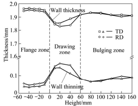
**Fig. 4** Distributions of wall thickness and wall thinning (thickness reduction) of deformed semispherical part
