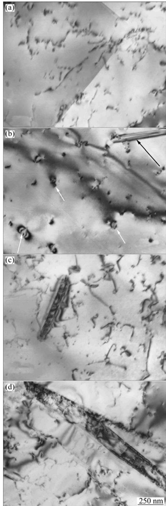
**Fig. 7** TEM images in BZ: (a) Dislocations at grain boundary; (b) Dislocation loops (at white arrows) and stacking fault (at black arrow); (c) Twin and dislocations within a grain; (d) Twins at grain boundary
