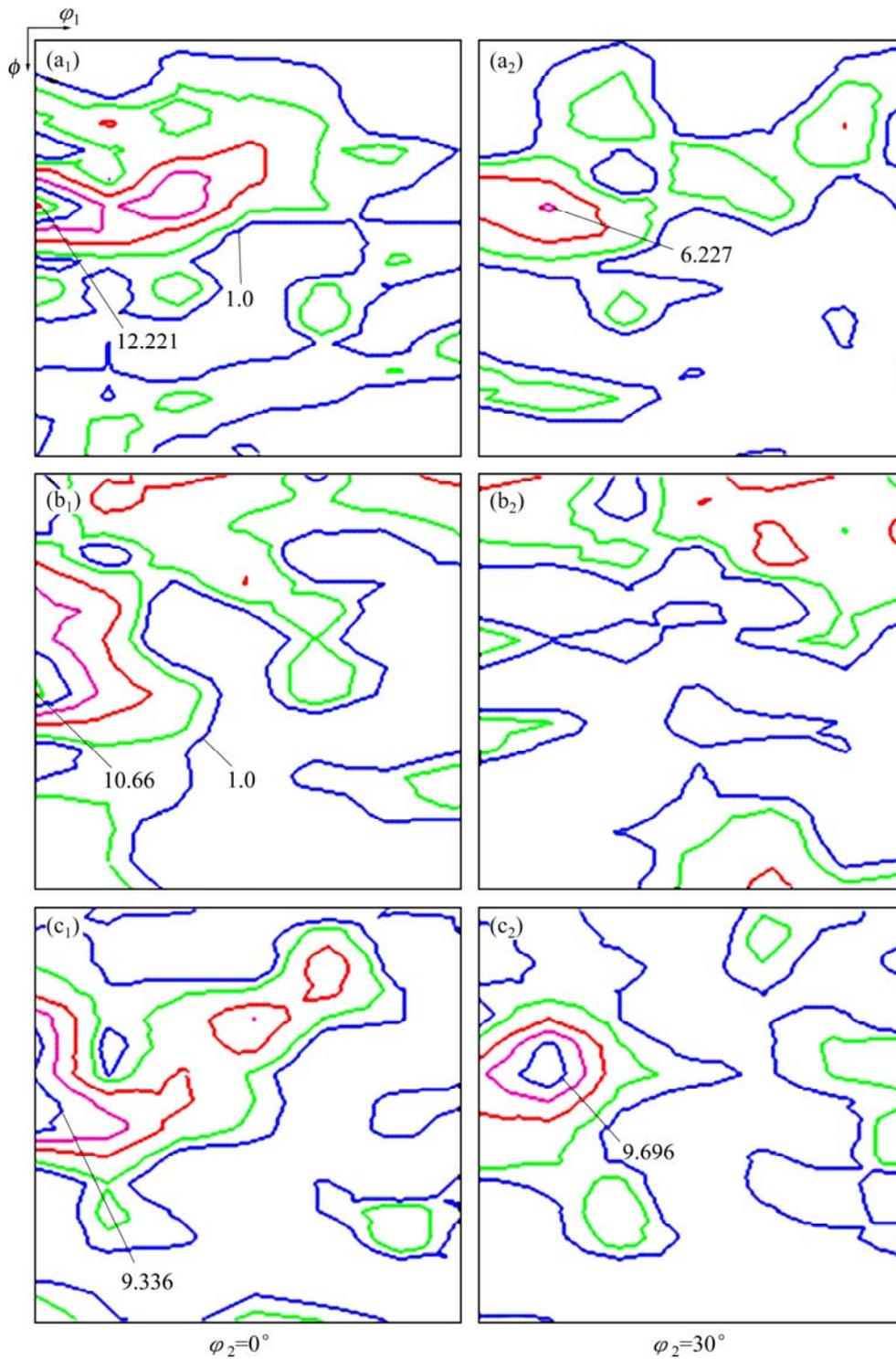
**Fig. 5** ODF sections of samples in BZ (a<sub>1</sub>, a<sub>2</sub>), DZ (b<sub>1</sub>, b<sub>2</sub>) and FZ (c<sub>1</sub>, c<sub>2</sub>) of finished part
