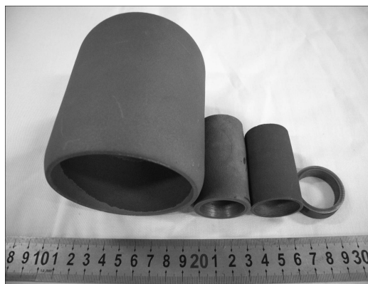
图 4 等离子喷涂近净成形 95W-3.5Ni-1.5Fe 薄壁回转体 Fig. 4 Near-net-shape of 95W-3.5Ni-1.5Fe thin-walled products fabricated by PSF
