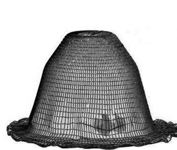
Fig.7 FE model for spinning of parts with inner rib and groove of mandrel
