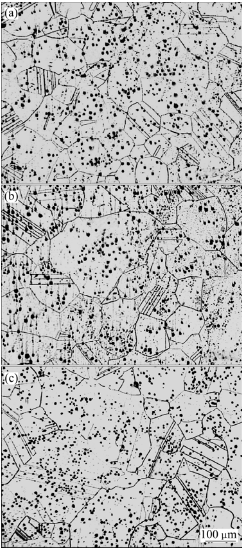
图 2 1 280 ℃ 下 MIM Fe-50%Ni 试样烧结不同时间的金相组织 Fig.2 Metallographs of MIM Fe-50%Ni specimens sintered at 1 280 ℃ for different sintering times: (a) 2 h; (b) 6 h; (c) 10 h
