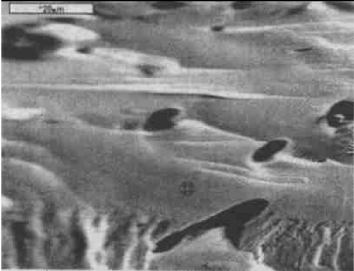
图 3 试样断口解理刻面的测试点 Fig. 3 Marked point location for EBSD on fracture surface of bending fractured specimen
