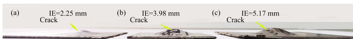
Fig. 14 Erichsen test (IE) values of various thermally-rolled AZ31 alloy sheets under annealed conditions: (a) Conventionally hot-rolled sample; (b) Sample A4; (c) Sample B4
