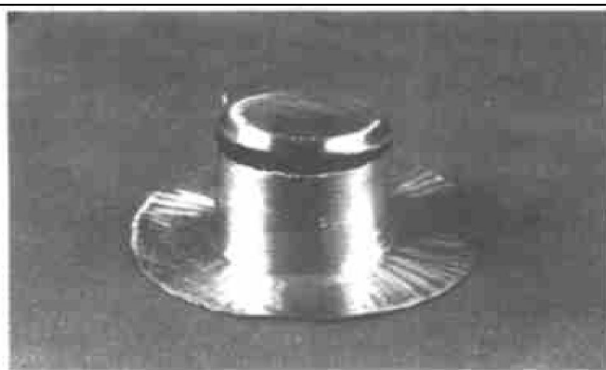
Fig. 7 Fracture caused by low punch temperature
