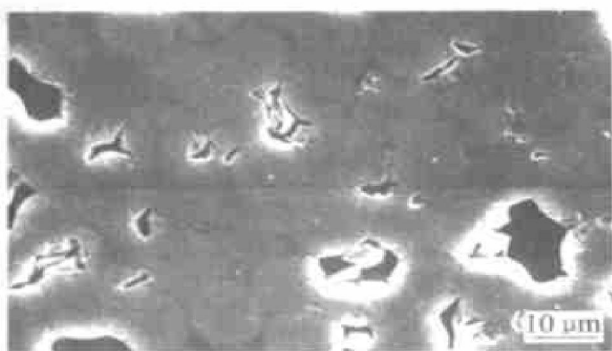
图 4 样品的残留孔洞 Fig. 4 Residue pores of specimens
