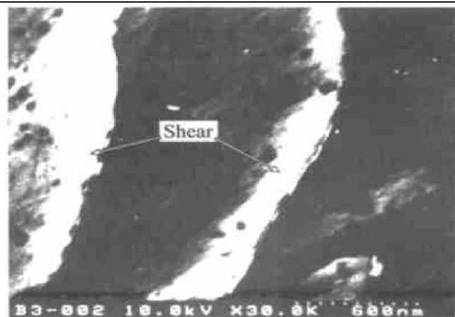
Fig. 2 Multiple circular pile-up around indentation
