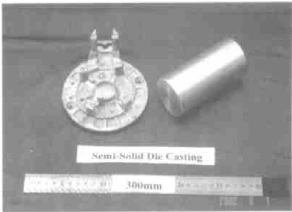
图 9 半固态铸造成形的 JH70 型摩托发电机支架 Fig. 9 Component used in JH70 motors formed by semi solid die casting processing
