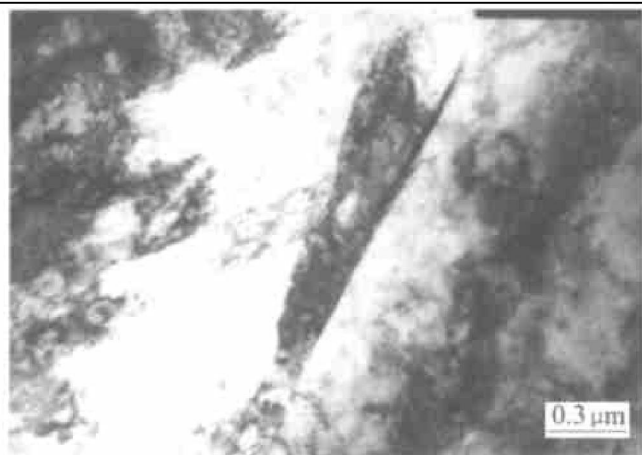
Fig. 9 Microstructure in intensive plastic deformation zone at stress of 368 MPa
