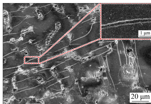
Fig. 5 SEM image showing corrosion morphology of MgZn 0.5 Y 0.67 alloy after immersing in 3.5 wt.% NaCl solution for 30 min
