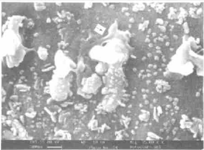
图 4 TiC/Ti 激光熔覆层中初生 TiC 形貌 Fig. 4 Morphology of primary TiC particle in TiC/Ti composite coating
