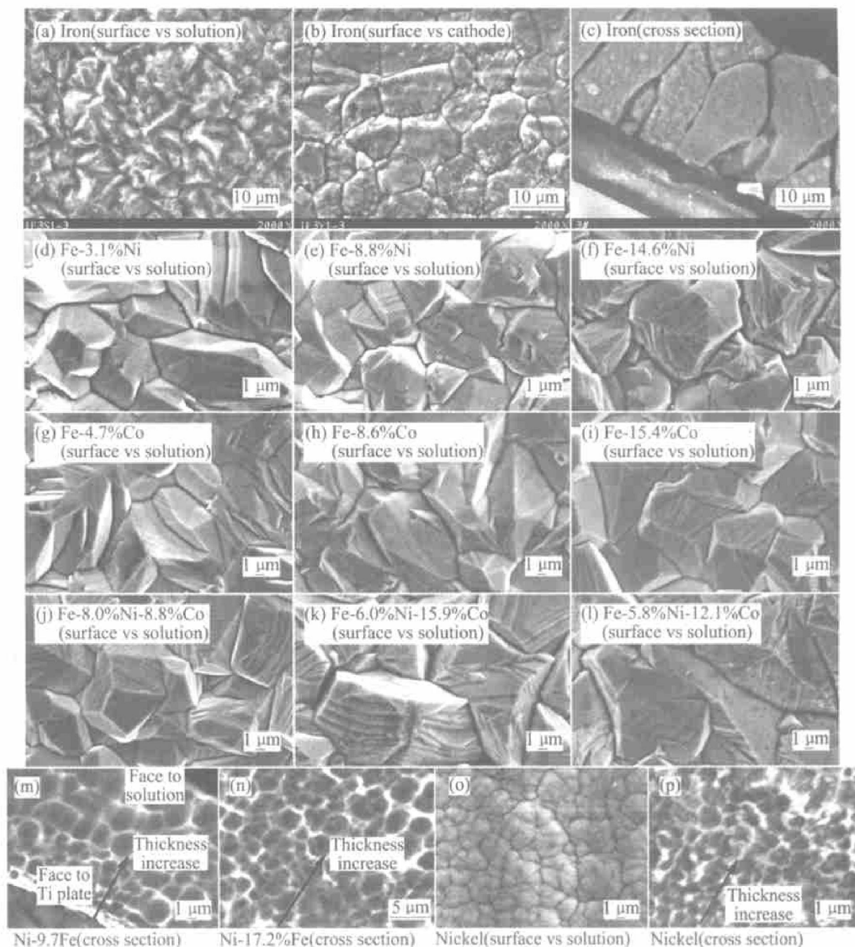
图 2 电沉积铁、镍基合金箔的组织形貌 Fig. 2 SEM images of electrodeposited iron and nickel based foils
