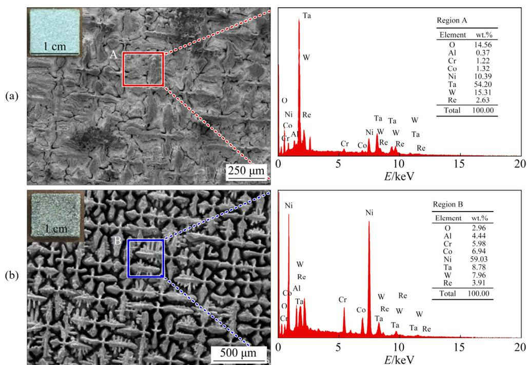
**Fig. 5** SEM images and EDS analysis results of superalloy scrap by normal (a) and ultrasonic-assisted (b) leaching process
