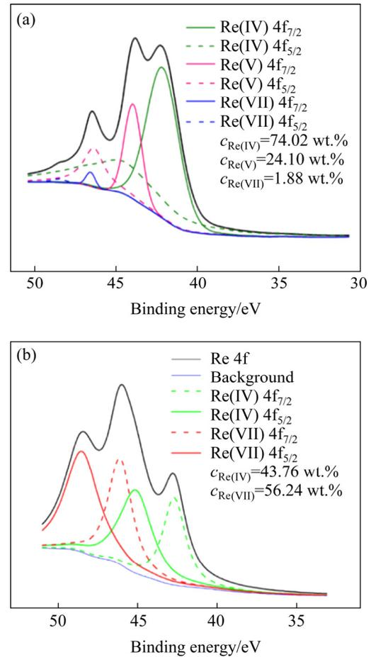
**Fig. 7** XPS analysis results of leaching solution by normal (a) and ultrasonic-assisted (b) leaching
