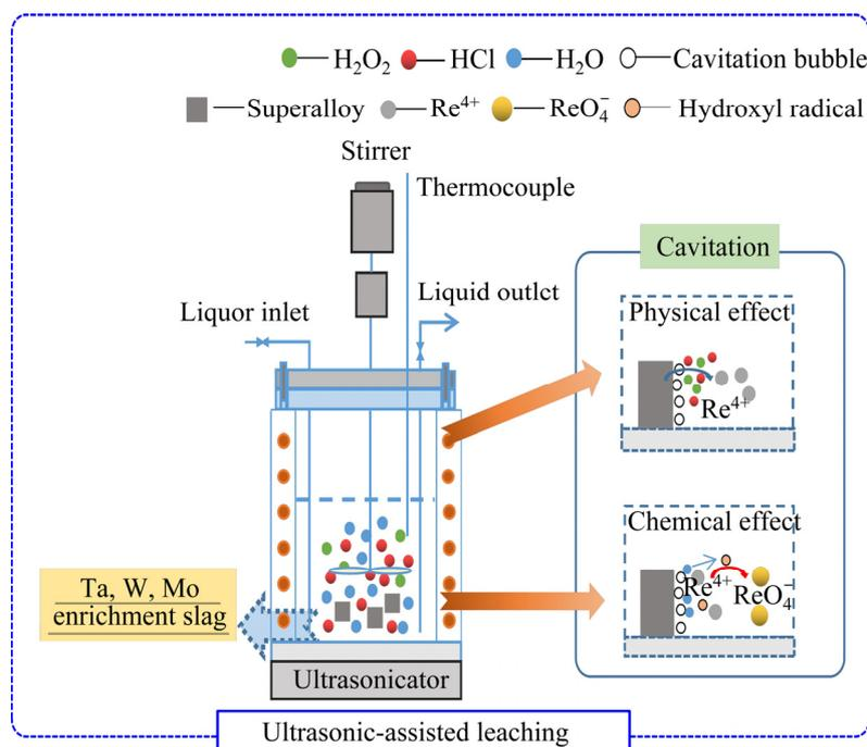
**Fig. 2** Schematic diagram of leaching experiment device
