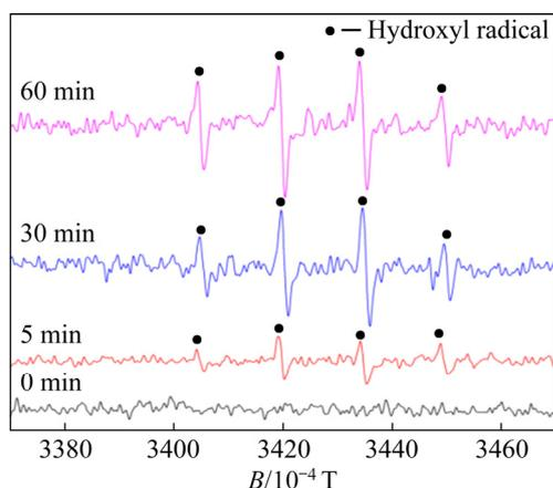
**Fig. 8** EPR spectra for hydroxyl radical determination in HCl–H<sub>2</sub>O<sub>2</sub> system at different leaching time in ultrasonic-assisted leaching process
