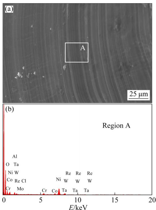
**Fig. 1** SEM image (a) and EDS analysis (Region A) (b) of superalloy scrap
