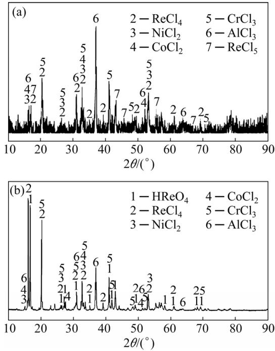
**Fig. 6** XRD patterns of leaching solutions by normal (a) and ultrasonic-assisted (b) leaching
