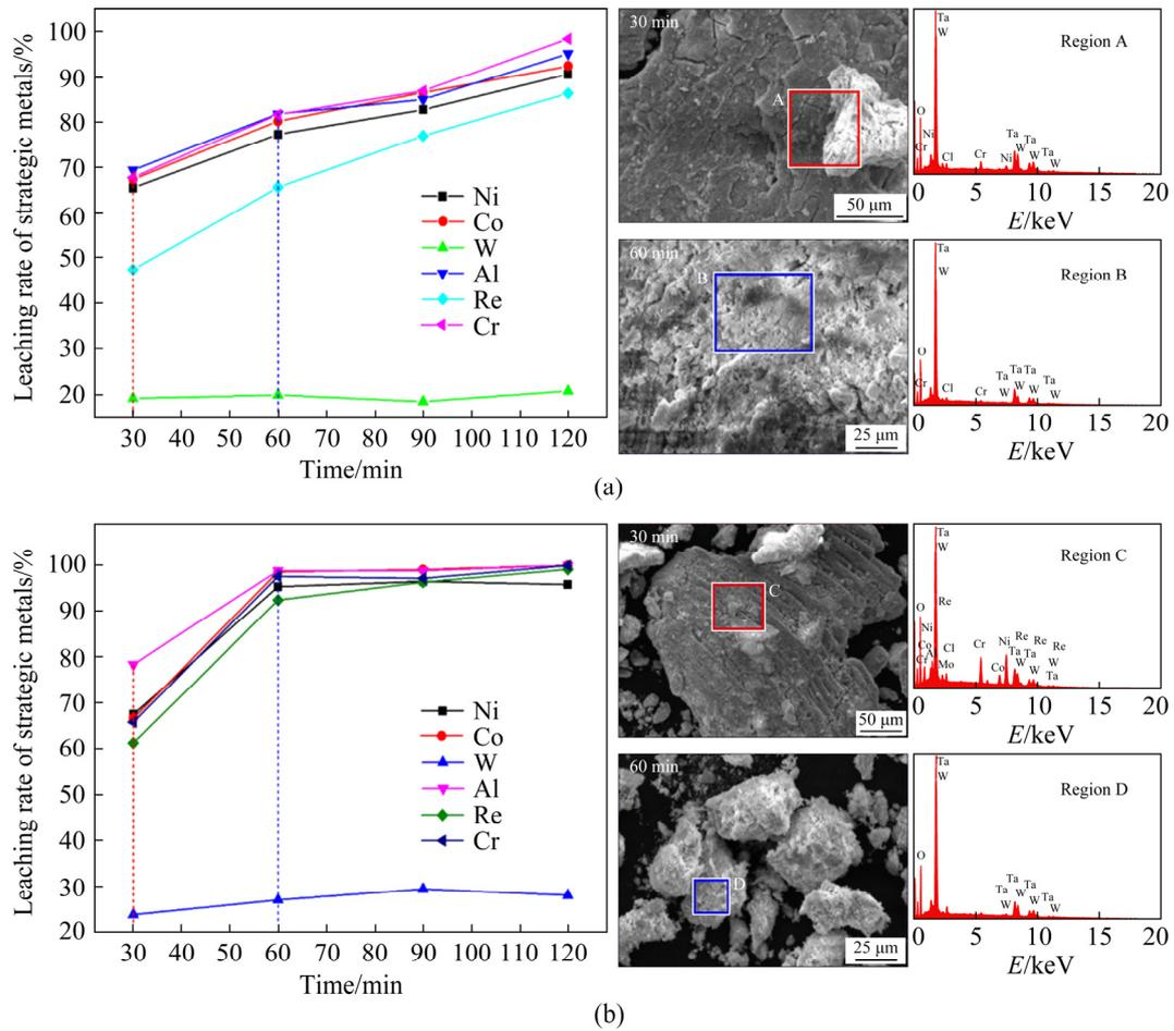
**Fig. 3** Leaching rates of strategic metals from superalloy scrap, SEM images and EDS analysis of leaching residues at different time with different leaching processes: (a) Normal leaching; (b) Ultrasonic-assisted leaching
