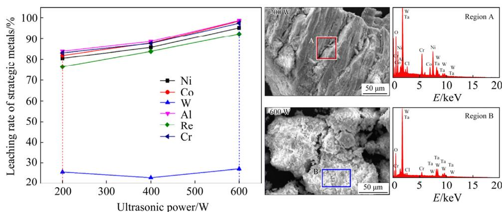
**Fig. 4** Leaching rates of strategic metals from superalloy scrap, SEM images and EDS analysis of leaching residues at various ultrasonic powers in ultrasonic-assisted leaching
