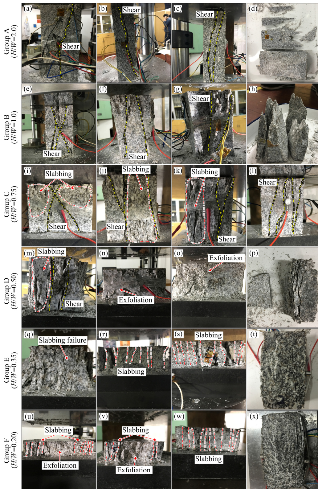
Fig. 5 Typical failure results of some specimens in Groups A (a–d), B (e–h), C (i–l), D (m–p), E (q–t) and F (u–x)
